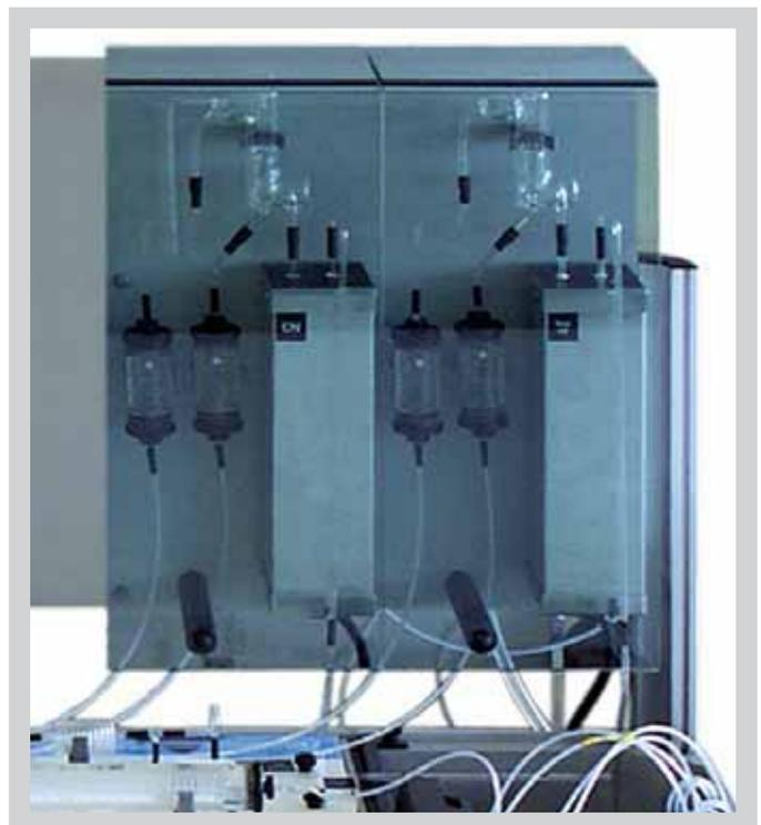
Two continuous thin film distillation set-ups
