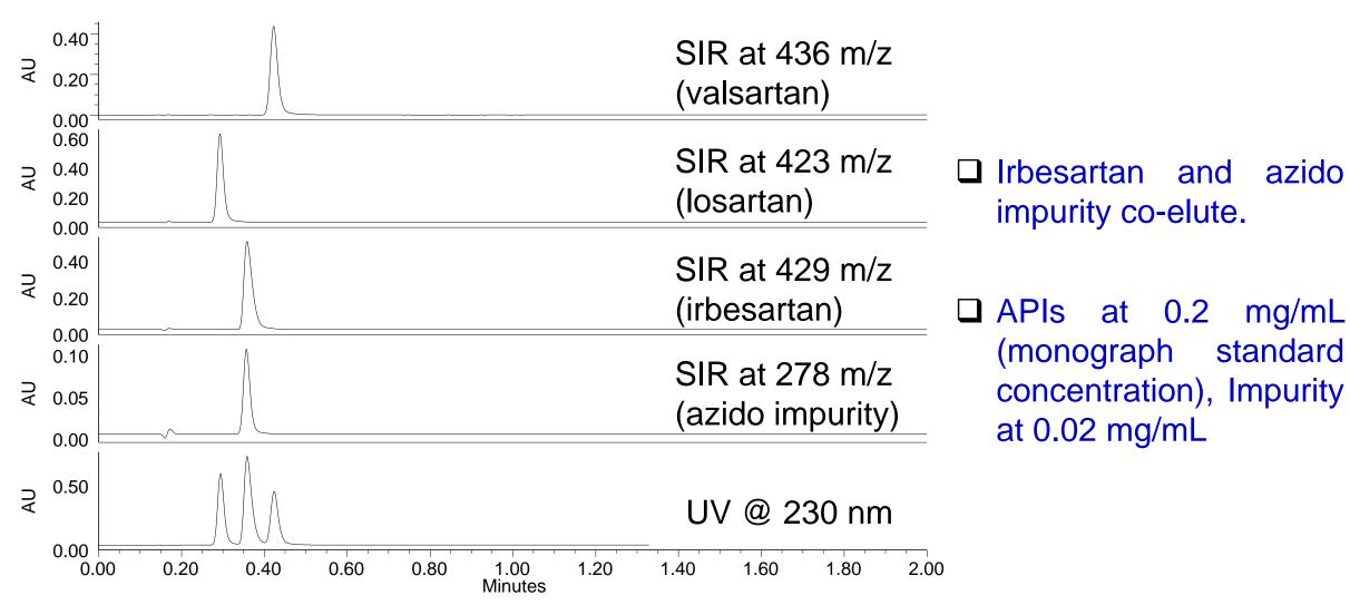
Assay conditions: XBridge BEH C18 (3.0 x 50 mm; 2.5 µm), Acetonitrile – Water - Acetic Acid (50:50:0.1), 1.7 mL/min
