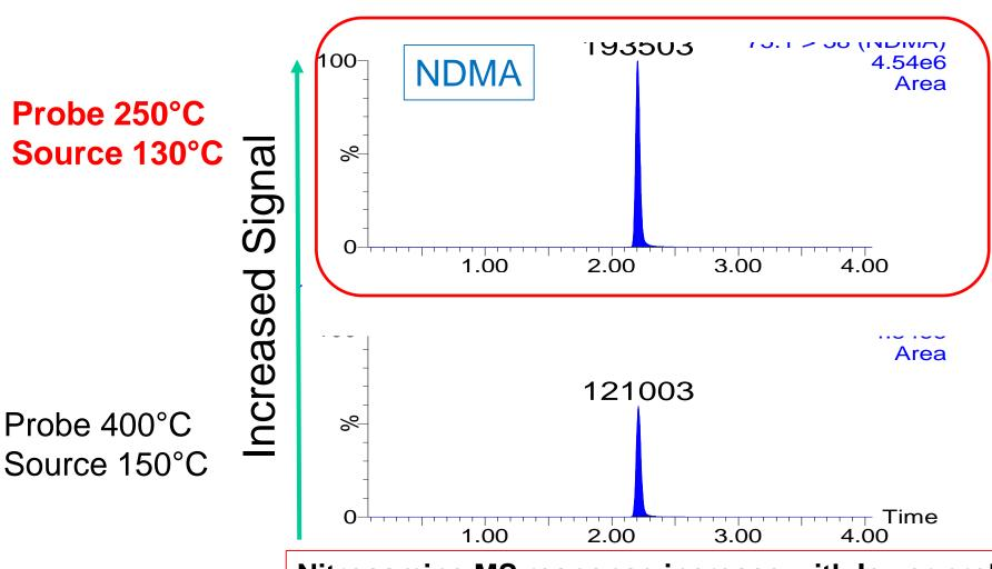
Nitrosamine MS response increase with lower probe and source temps
