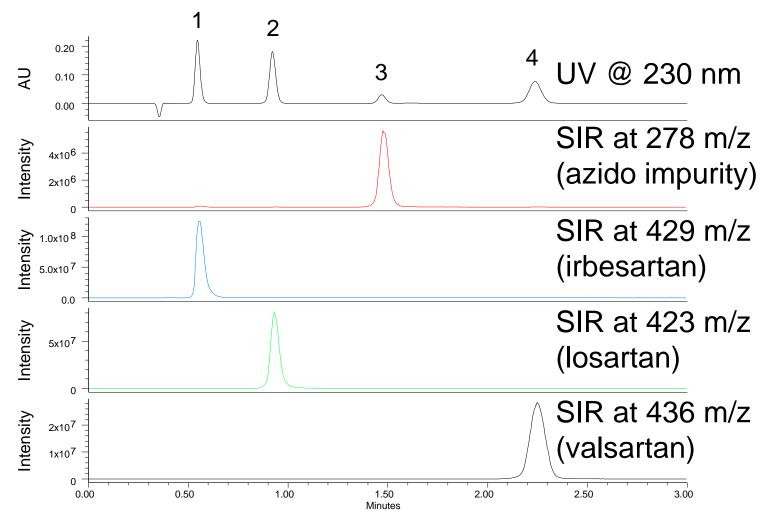
40% acetonitrile with 0.1% formic acid, 0.85 mL/min, 30°C, XSelect CSH Phenyl-Hexyl (3.0 x 50 mm; 2.5 μm)
